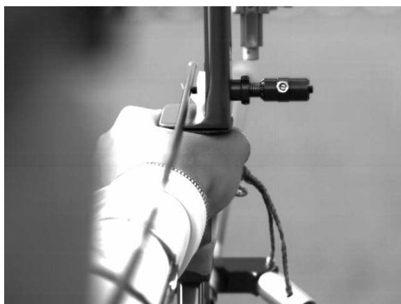
Arrow pushes against Plunger, moving plunger in about .5 mm
