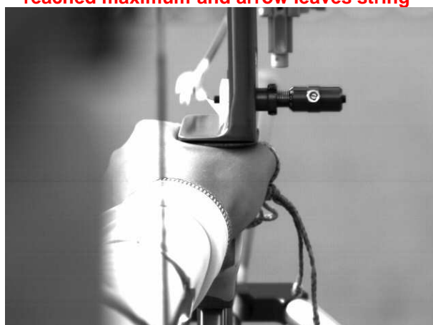
Arrow passes arrow rest without contact
