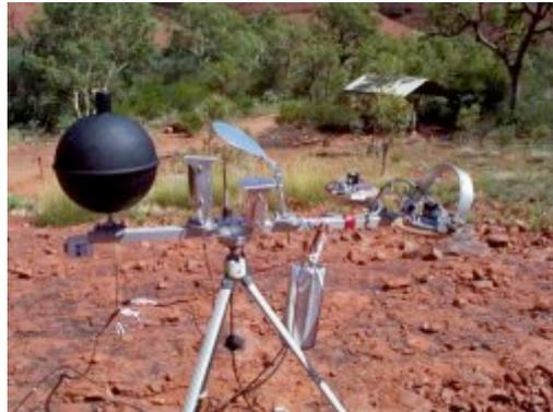
The **WBGT** was later used by researchers as an easily measured general heat-stress index. In time its use widened. Because its use is recommended in the Standard, ISO 7243, it is often used in Occupational Health and Safety guidelines for working in hot environments. It has been advocated for use in sports requiring continuous exertion, such as the marathon. It is also used for horses in equestrian events.
